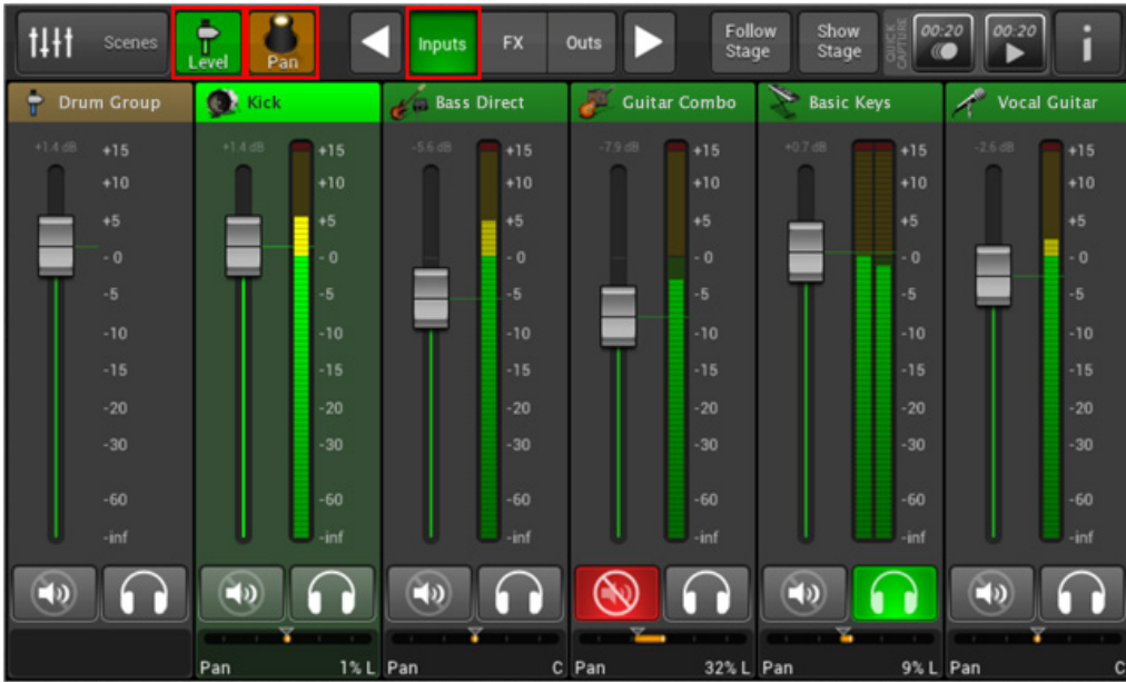
Perform mode: Fader View in Inputs Select mode (with Level and Pan assignments)
